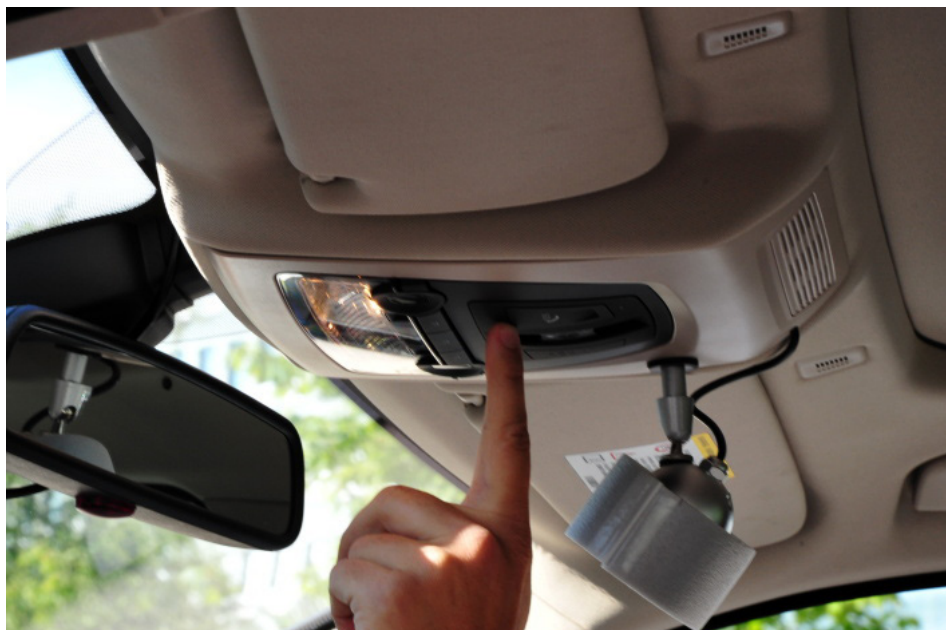
Pict. 2. Manual SOS button in a BMW car for communication with a Public single answering point (PSAP)
